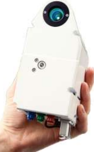
Rikola FPI – VNIR 2D Hyperspectral sequential imager (Honkavaara et al., 2013)
