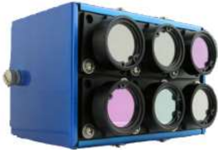
TetraCam mini-mca Multispectral 2D imager (Berni et al., 2009) (Kelcey and Lucieer, 2012)
