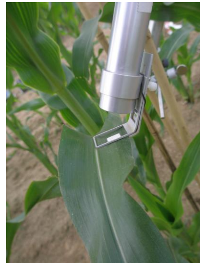
Fig. 2c - Details of the sample holder with corn leaf
