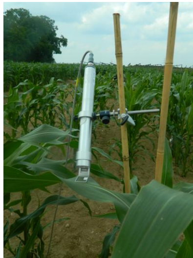
Fig. 2b - MONI-head emitter-detector unit in a installation at the top leaf
