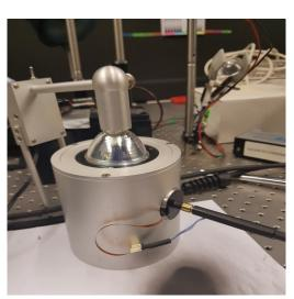
Figure 7 TH lamp aligned with hyperspectral sunphotometer integrating sphere fore optic and with spectrometer fibre optic attached.
