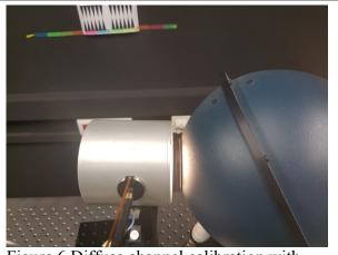
Figure 6 Diffuse channel calibration with LEO integrating sphere
