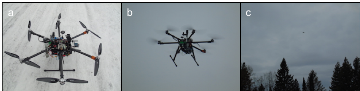
Figure 2 | The test flight of the Piccolo Doppio aboard the UAV. The fibre optic heads of the Piccolo system can be seen on the left hand side of the UAV in (a). The system in the air (b) and above the trees (c).
