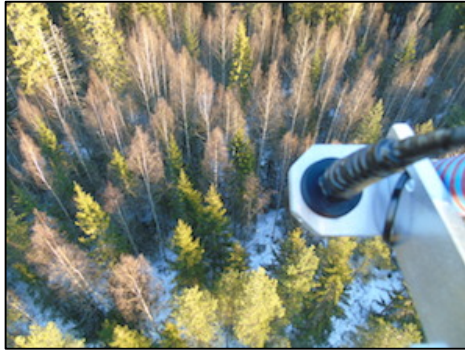
Figure 3 | the tower-based Piccolo Doppio system and field of view, showing evergreen pine and spruce and deciduous birch with snow background
