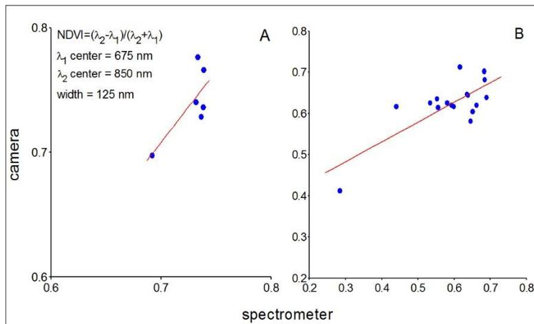
Fig. 13. Correlation between camera-derived and spectrometer-derived NDVI for wavebands providing to the least deviations between these parameters. A – ground experiment; B – airborne experiment
