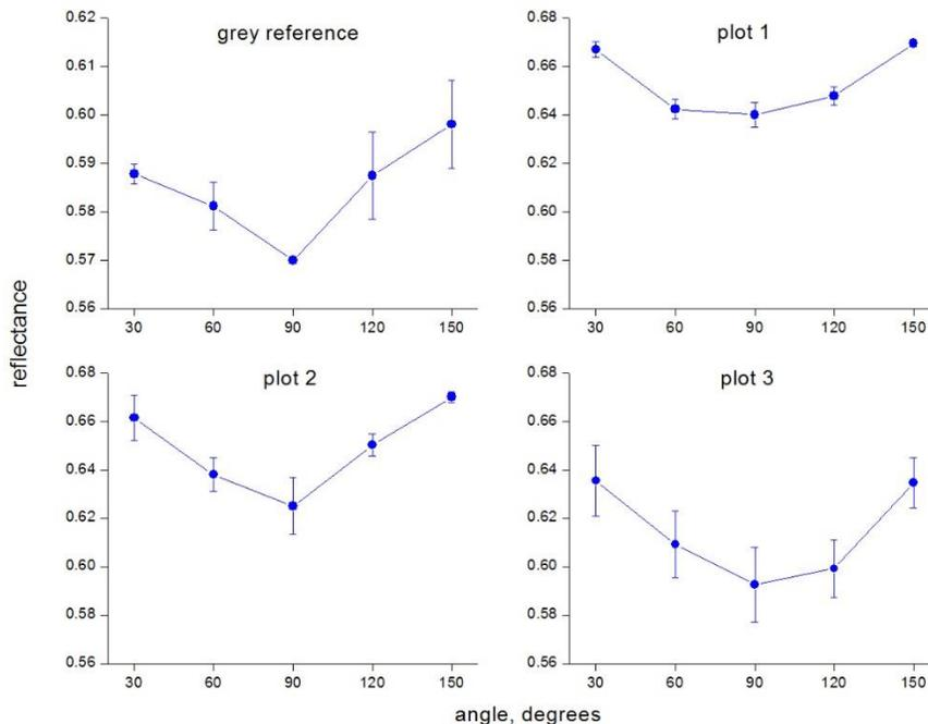
Fig. 11. Effect of observation angle (to horizon) on signal in NIR band of camera
