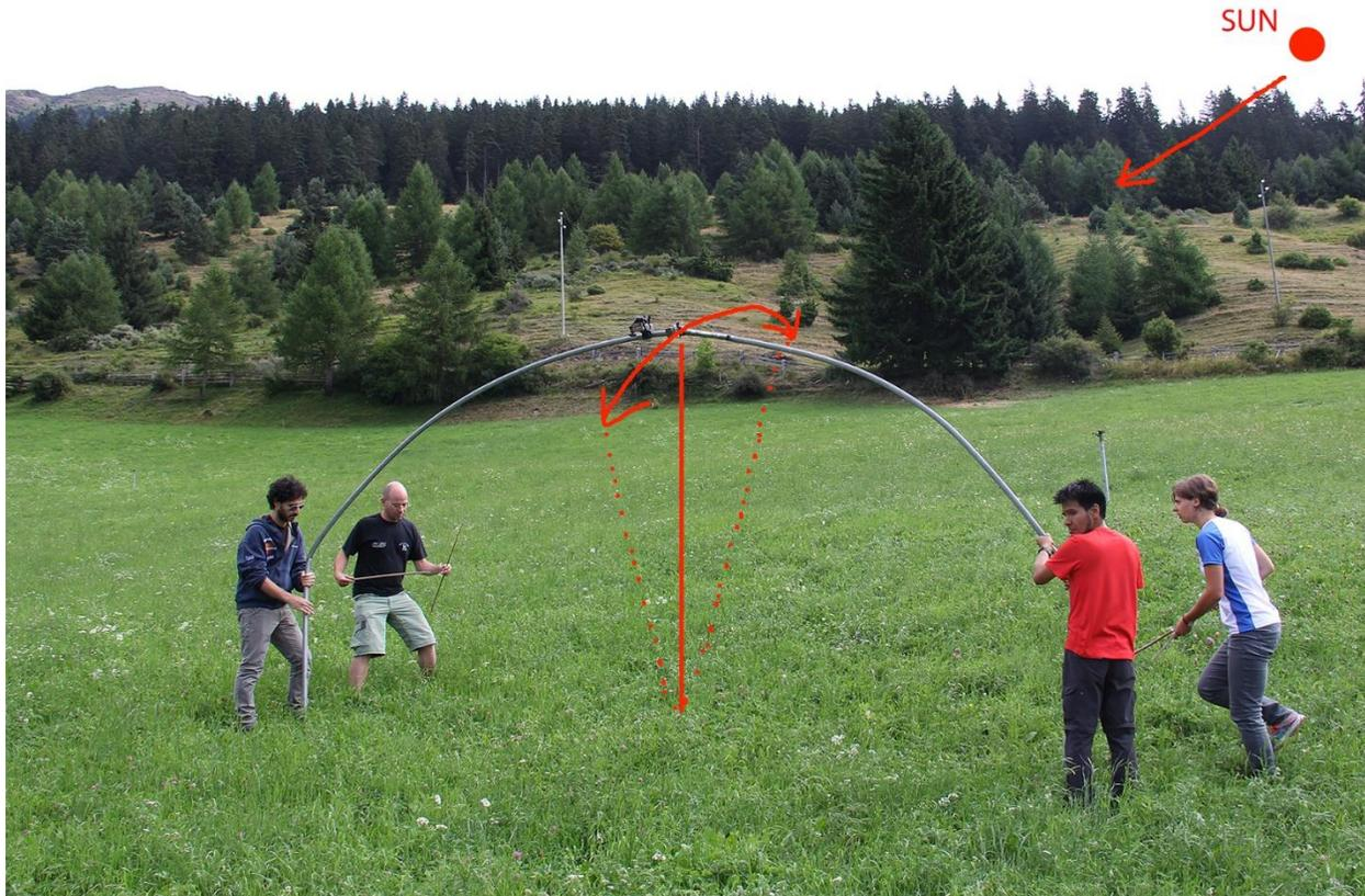
Fig. 2. Scheme of capturing images under different angles (studying BRDF effects)
