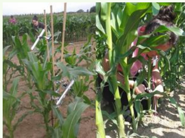
Chiara's experimental setup. On the left: Moni-PAM units sampling maize leaves located at different canopy layers. On the right: Fluowat measurements of bottom maize leaves.
