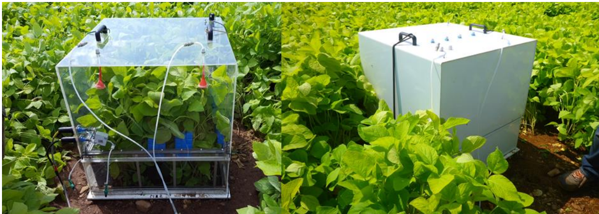
Image 5. Chamber NEE (left panel) and Reco (right panel) measurements.
