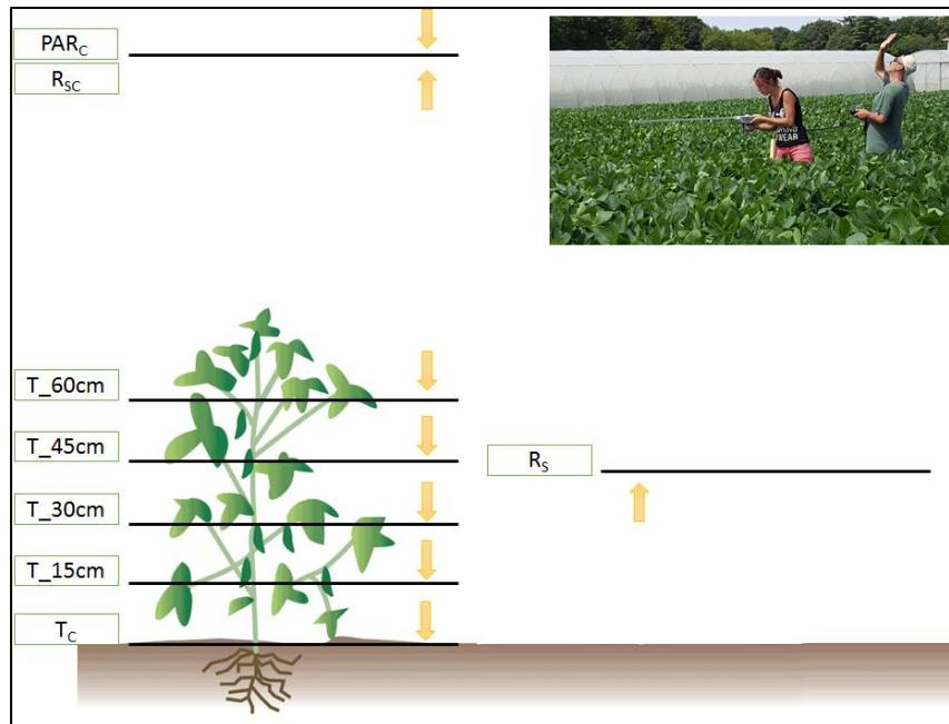
Image 6. Sensor configuration for along-row measurement of i) FAPAR_{canopy} and ii) PAR transmitted at different canopy heights ( T_C \dots T_{60cm} ). Sensors facing upward when measuring downward PAR_C and T, and downward when measuring upward R_S and R_{CS} .
