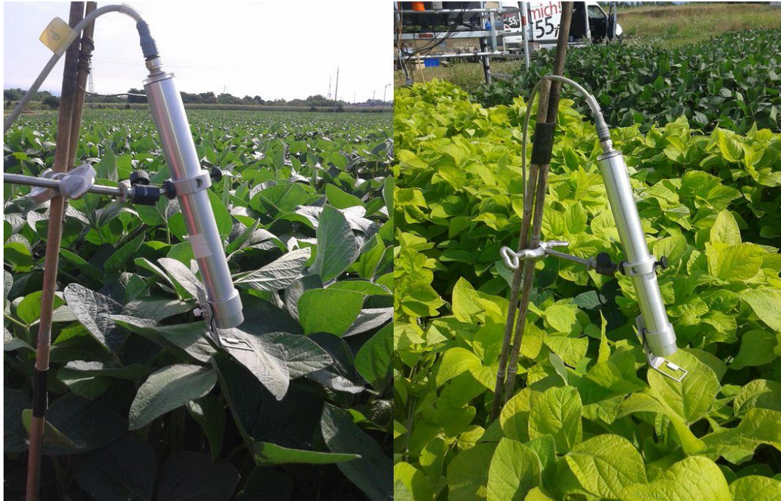
Image 2. Moni-PAM head emitter-detector unit sampling the top leaves of Eiko (left) and Minngold (right) soybean plants.
