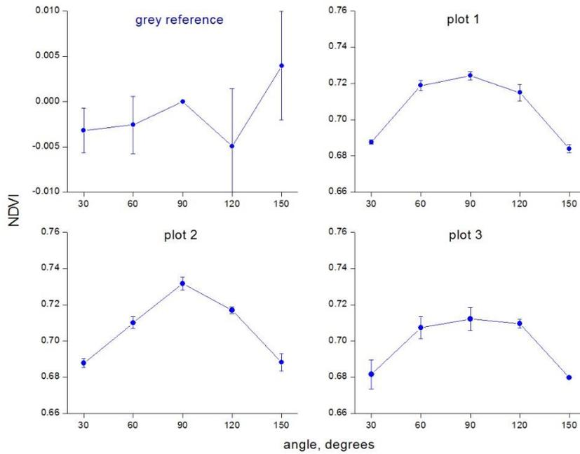
Fig. 12. Effect of observation angle (to horizon) on NDVI
