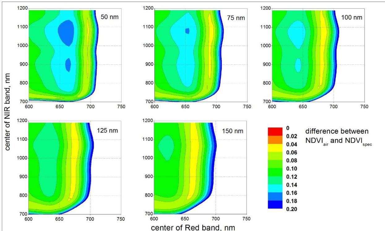
Fig. 8. Deviation between camera-derived NDVI (from air) and spectrometer-derived NDVI calculated with different wavelengths. X and Y axis = centers of wavebands; width of wavebands indicated in the right upper corner.
