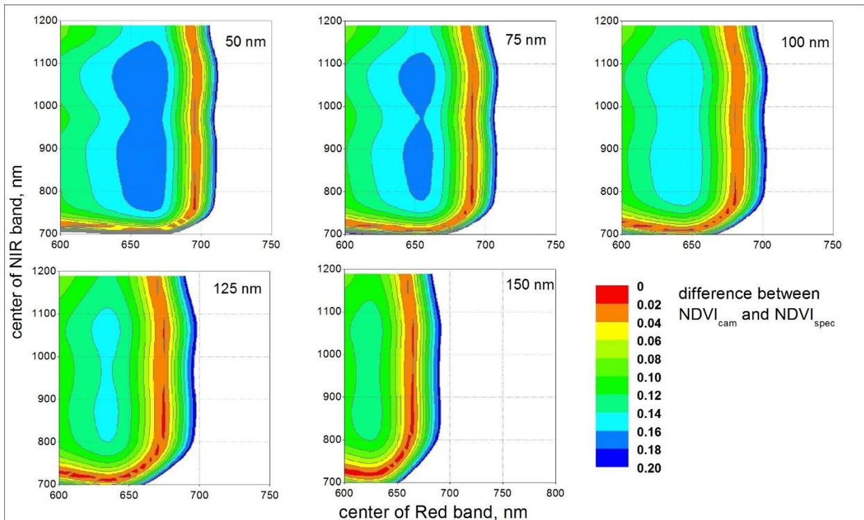
Fig. 6. Deviation between camera-derived NDVI (from ground) and spectrometer-derived NDVI calculated with different wavelengths. X and Y axis = centers of wavebands; width of wavebands indicated in the right upper corner.
