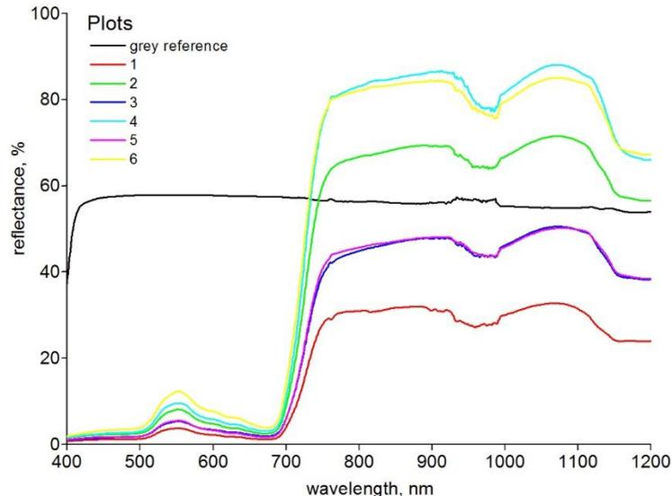
*Fig. 5. Reflectance spectra of vegetation plots used for comparison of readings from cameras and spectrometer.*
