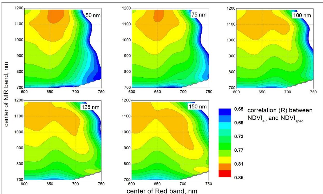
Fig. 9. Correlation between camera-derived NDVI (from air) and spectrometer-derived NDVI calculated with different wavelengths. X and Y axis = centers of wavebands; width of wavebands indicated in the right upper corner.
