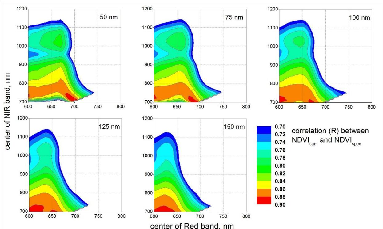
Fig. 7. Correlation between camera-derived NDVI (from ground) and spectrometer-derived NDVI calculated with different wavelengths. X and Y axis = centers of wavebands; width of wavebands indicated in the right upper corner.
